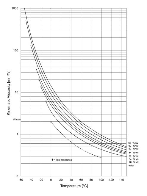
Kinematic Viscosity of Antifrogen N - water mixtures of different concentrations
