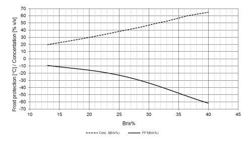
Frost protection / Concentration of Antifrogen N - water mixtures in response of the nD20
