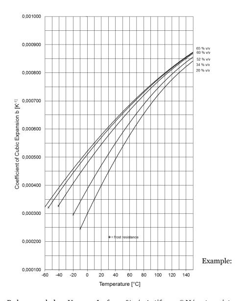
By how much does  $V_o = 100 \text{ L}$  of a 35 % v/v Antifrogen® N/ water mixture expand on heating from  $t_o = -10$  °C to  $t_1 = 80$  °C?  $\Delta_t = t_1 - t_0 = +80 - (-10) = 90$ °C  $t_{average} = t_0 + \frac{\Delta t}{2} = -10 + \frac{90}{2} = 35$ °C  $\beta t_{average}$  (from the curve for 35 % v/v = 0,00051  $\Delta V = \beta t_{average} * \Delta t * V_0 = 0,00051 * 90 * 100$ = 4,6 L increase in volume
