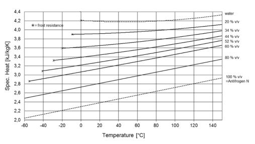
Specific Heat of Antifrogen N - water mixtures of different concentrations
