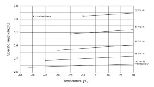
Specific Heat of Antifrogen KF-water mixtures of different concentrations
